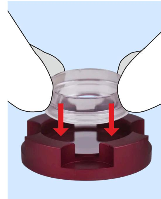
**8** Position the dish, adhesive-/bottom face down, in to the center of the Glass-Holder and press firmly. This will create a strong bond between the pressure sensitive DSA adhesive and the glass coverslip.
