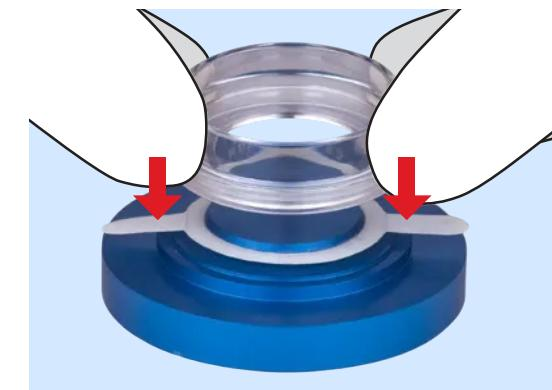
**3** Position the opening in the bottom of the dish (right type!) over the same notch in the center of the Adhesive-Holder and press the dish down, firmly.
