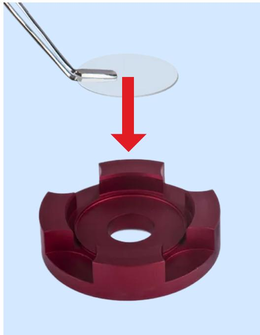
**6** Using the tweezers, position the glass coverslip within the outer wall of the glass-holder and carefully shuffle the holder between your fingertips, to make the glass coverslip slide gently into place in the center of the chamber.
