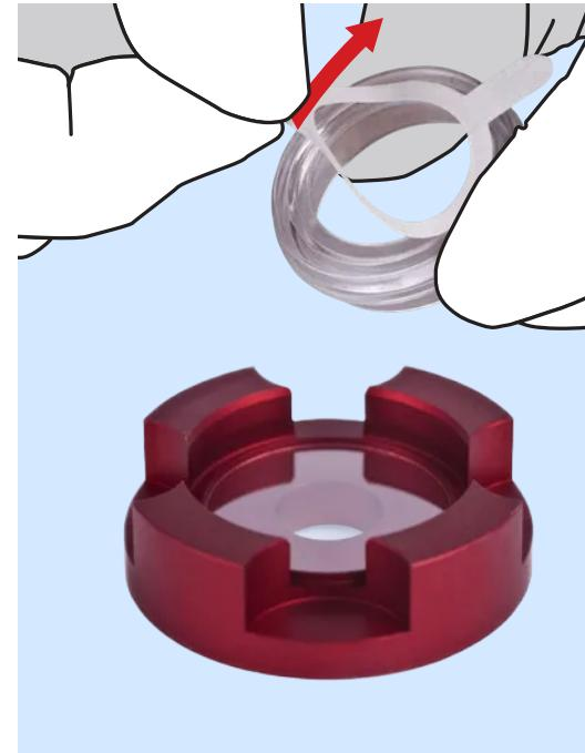
**7** Only now, take off the white adhesive liner/carrier from the bottom of the dish, by gently pulling of the "easy peel" slip.
