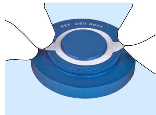
**2** Position the opening in the white adhesive liner/carrier, **adhesive facing up**, over the round center notch on the **"Adhesive-Holder"**, to rest on the base.
