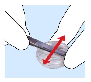
10 Check the bonding along the whole adhesive area and again look for air-pockets. It is natural to have these air-pockets, which are easily removed by putting little pressure on the glass, using the flat back-end of the tweezers.
