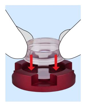
8 Position the dish, adhesive-/bottom face down, in to the center of the Glass-Holder and press firmly. This will create a strong bond between the pressure sensitive DSA adhesive and the glass coverslip.
