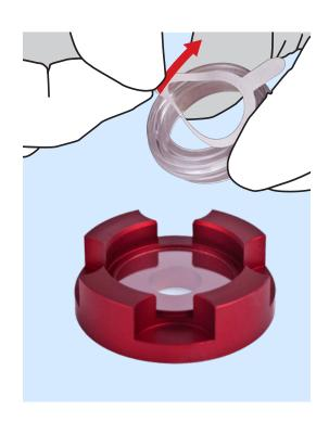
Only now, take off the white adhesive liner/carrier from the bottom of the dish, by gently pulling of the "easy peel" slip.
