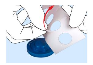
1 Take the white easy-peel adhesive liner off from the long liner-strip. **Note:** In case the adhesive ring does not release from the long liner-strip, then place the liner-strip over the Adhesive-Holder, adhesive ring face up.
