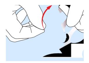
Take the white easy-peel adhesive liner off from the long liner-strip. Note: In case the adhesive ring does not release from the long liner-strip, then place the liner-strip over the Adhesive-Holder, adhesive ring face up.
