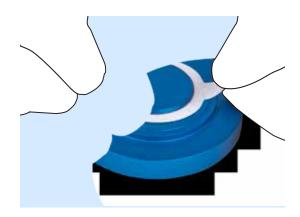
Position the opening in the white adhesive liner/carrier, adhesive facing up, over the round center notch on the "Adhesive-Holder", to rest on the base.
