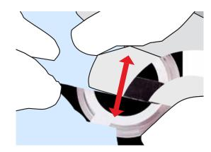
4 Take the dish from the Adhesive-Holder and check for small air-pockets. If necessary, finish the primary bonding by using only a little pressure with the round back-end of the tweezers.
