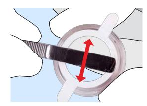
4 Take the dish from the Adhesive-Holder and check for small air-pockets. If necessary, finish the primary bonding by using only a little pressure with the round back-end of the tweezers.
