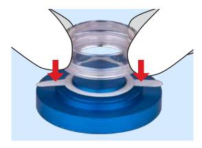
3 Position the opening in the bottom of the dish (right type!) over the same notch in the center of the Adhesive-Holder and press the dish down, firmly.
